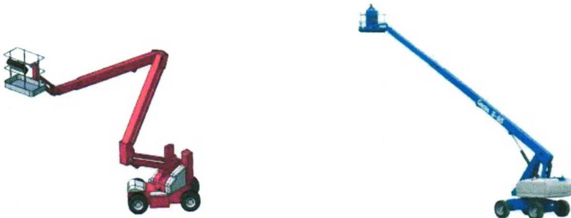
Self-propelled booms which can be driven when elevated. The 3b category includes articulated booms (which give 'up-and-over' outreach), and telescopic booms (which give 'line-of-sight' outreach).
