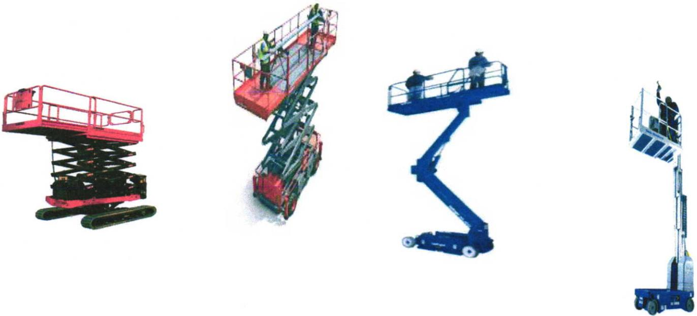
Self-propelled machines capable of vertical lift only (no significant outreach). Larger machines may have a maximum height restriction for driving - above this limit jacks need to be deployed which will prevent them from being driven along the ground (though these MEWPs are still classed as 3a machines). 3a machines can have scissor, sigma or vertical mast lift mechanisms.
