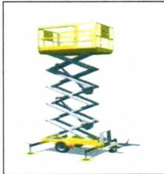
These static vertical systems are vertical personnel and mobile elevating work platforms (MEWPs) that can be driven into position from the working platform when in the stowed position. Before elevating, outriggers, jacks or stabilisers will need to be deployed, so this MEWP equipment cannot be moved along the ground when elevated.
